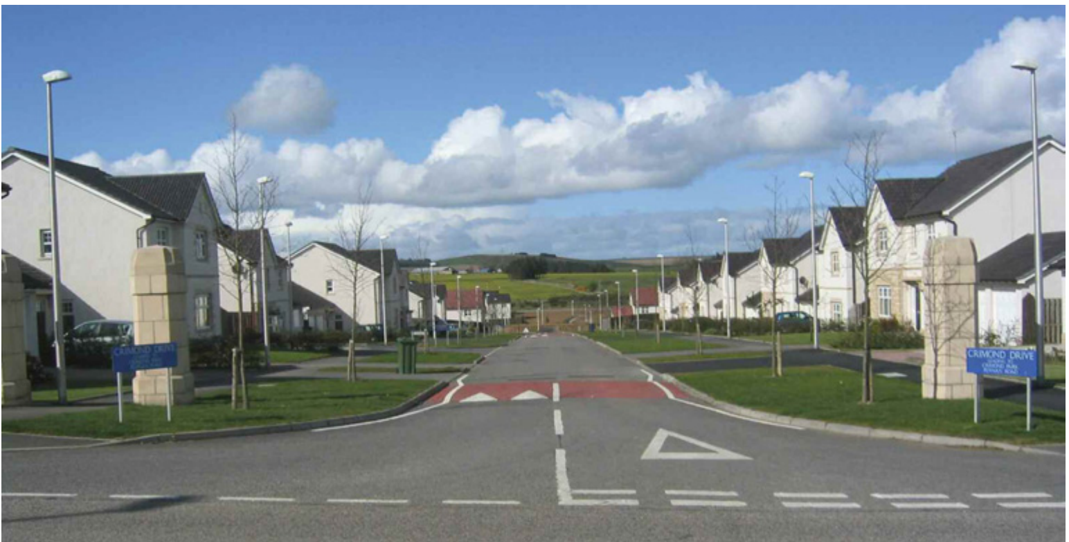
An image of a layout driven by standards and formulaic solutions – the use of large radius bends, overly-dominant lighting columns, large building setbacks, inefficient land use, and inappropriate traffic calming contribute nothing to a positive sense of place
